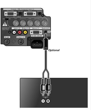
• Connect the Audio in L/R sockets of an amplifier or stereo system to the Audio out socket **(G)** of the projector. For this, use an audio connection cable **(optional)**.
